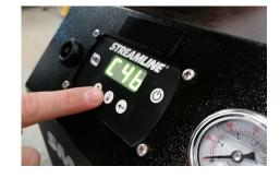
iv. Press 🚭 button to set and save the final calibration
