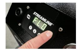
To adjust dead-end detection, press and hold and at the same time. Wait for 'Cal' to display and flash on the screen.
