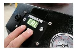
iii. When 'Cal' displays on the screen, adjust dead-end detection up with (less sensitive, turns off at higher pressures) or down with (more sensitive, turns off at a lower pressure).
