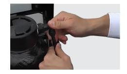
**iii.** Unscrew the filter bracket and remove the DI filter from the trolley.
