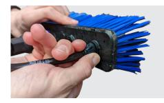
It is important to make sure there is a firm seal around the hose to help protect leakage. To make sure the hose is attached correctly when you push the hose into the tee-piece you should hear a click sound and then push it in a seccond time to make sure its fully secure. You can check by trying to pull the hose out the tee-piece.
