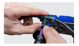
v. You can choose where you want your jets to be, which we place on the edge of the brush which you push your jet nozzles in and you simply twist and lock using the twist mechanisum, turning clockwise.
