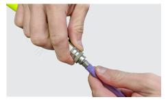
ii. Open up either your fan or pencil jets from the package or blister pack. In the pack there should be a tee-piece with a push fitting already attached. Using the tee-piece, make sure you push each one of the jets accessory into the John Guest tee-piece.
