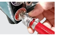
iv. Connect the BLUE hose from the pure water outlet to your water-fed pole (it is possible to add a Streamline® 100mtr hose reel)
