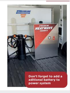
**HEATWAVE**™ water heater systems use diesel from either the vehicle's fuel tank or a separate remote tank that can be filled with red diesel for economy.
