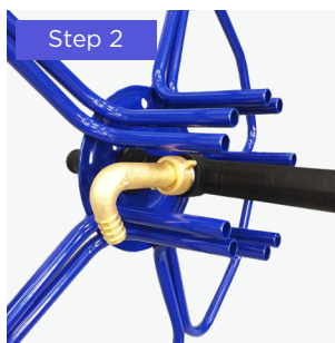
Step 2: Attach outlet elbow (E) to centre manifold (D) and tighten, remembering to insert washer behind the flynut.
