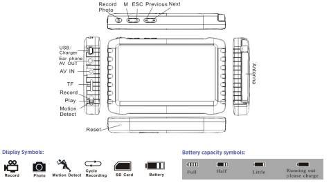
The possible reason for the Monitor not powering up, is that the battery is depleted. Plug the charging wire into the USB port on the monitor and connect it to a mains voltage supply.
