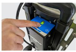
To check voltage of battery, press the controller button twice, voltage of battery will display. It is recommend any battery lower than 10.5v requires charging.
