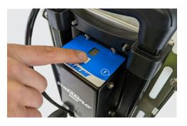
Now you can adjust the speed of the water flow through the 100psi multi-speed pump by pressing and holding the button on the flow controller untill you reach the desired setting
